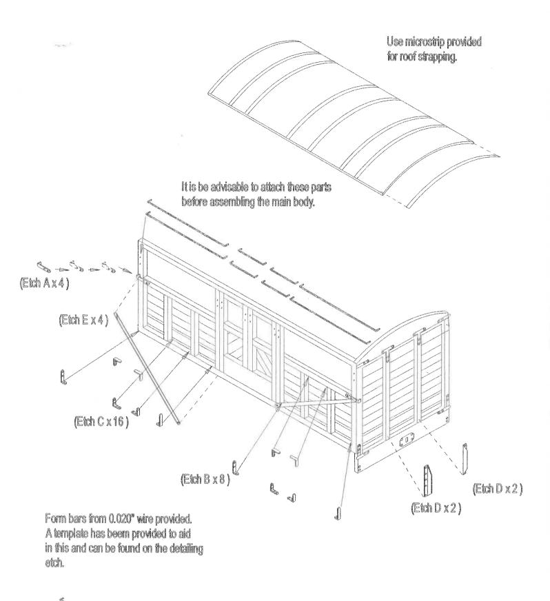
The bars are either 46.5mm or 15mm long with 2mm added for depth.
